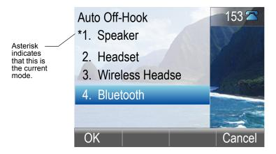
Step 4 Highlight the desired option and press the OK soft key.
