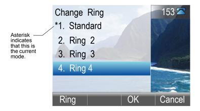
**Step 4** Press the OK soft key when you've chosen the ring you want, and press the **Done** soft key.
