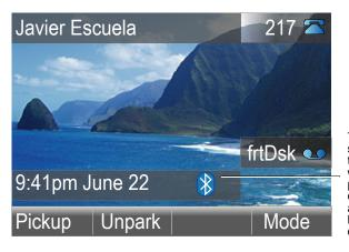
This symbol indicates successful pairing of the Bluetooth headset with your 565g IP phone. The symbol changes to grey (with a line through it) if the headset is powered off or is out of range.
